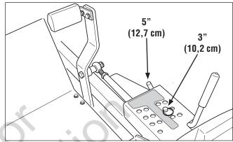
Figure 40. Deck Lift Pedal & Pin Position
